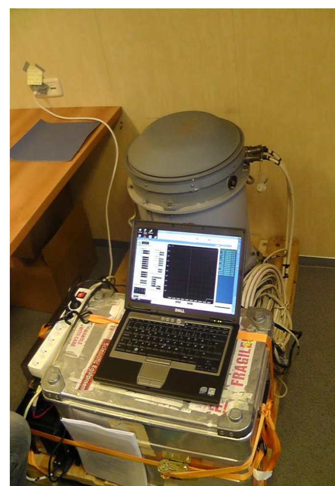
Fig. 6. Russian „Elektropribor” manufactured gravimeter Chekan-AM for marine gravimetric data acquisition (photo A. Ellmann).
